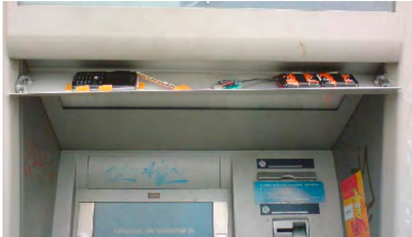
Figure 1 A modified teller machine (with a false cover for a slot for inserting the card and a hidden telephone used as a camera to record PIN).
